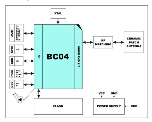
The Bluetooth module is a self-contained Bluetooth product and requires only power to implement full Bluetooth communication. The integrated, high performance antenna together with the RF and Base-band circuitry provides the Bluetooth wireless link and the UART interface provides a connection to the host system.
