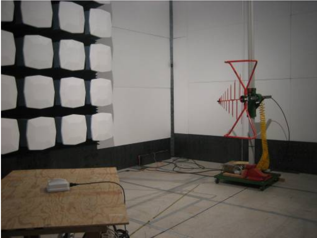
Radiated Emission 30MHz to 1GHz-
