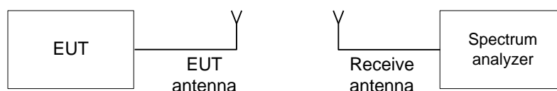
Figure 7.3.1 Occupied bandwidth test setup
