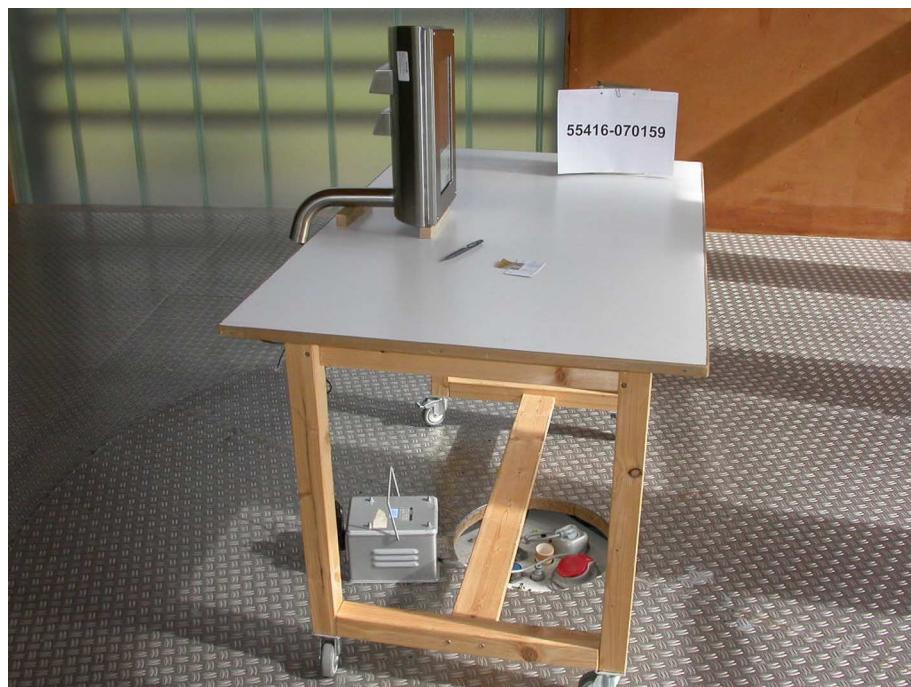
**Test setup for radiated emission measurement
