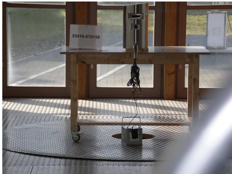
**Test setup for radiated emission measurement
