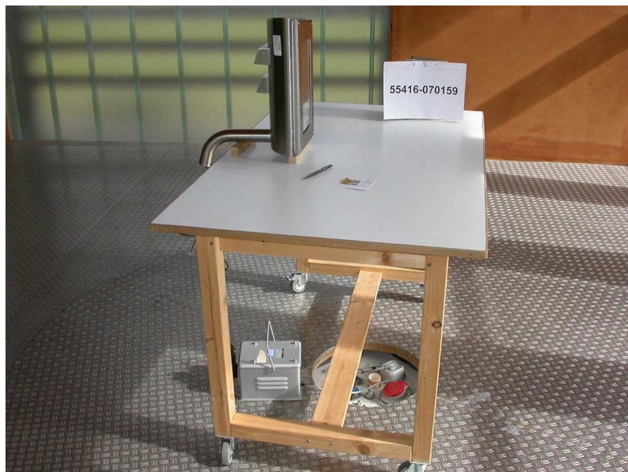
**Test setup for radiated emission measurement
