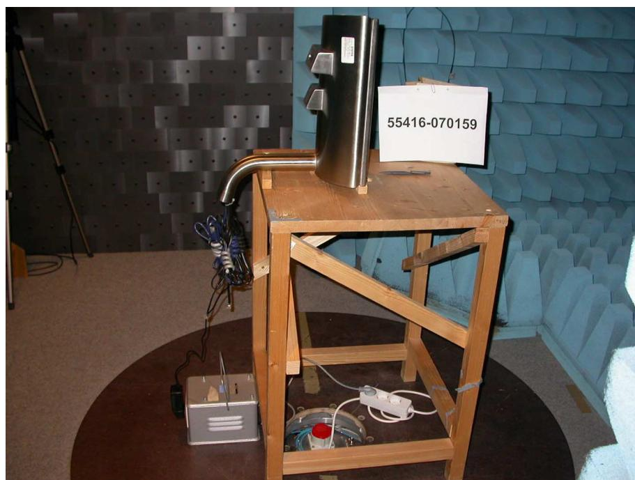
**Test setup for radiated emission measurement
