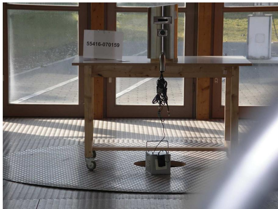
**Test setup for radiated emission measurement
