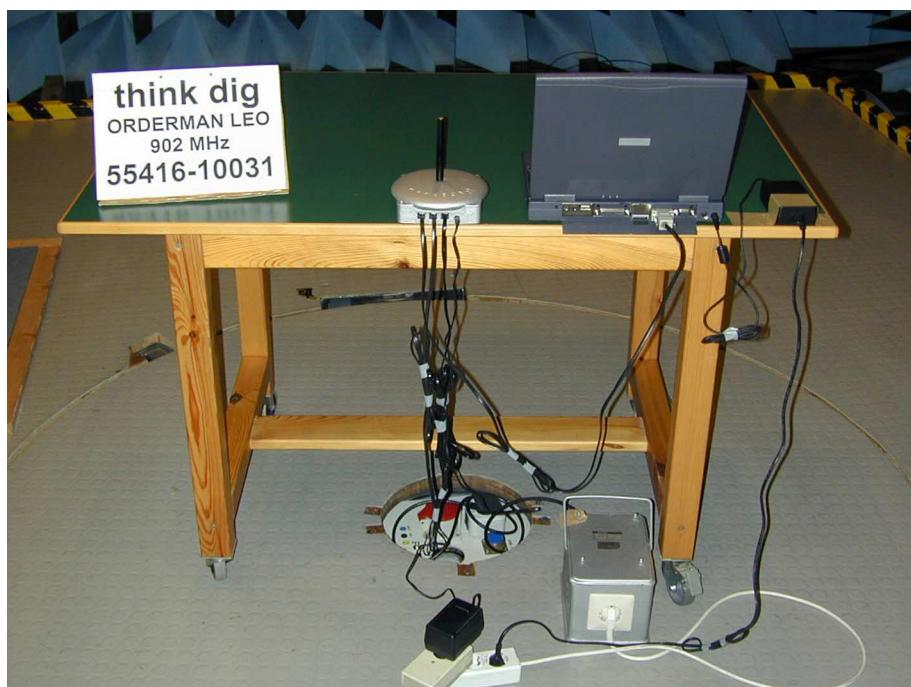
**Radiated Emission Measurement >30 MHz**
