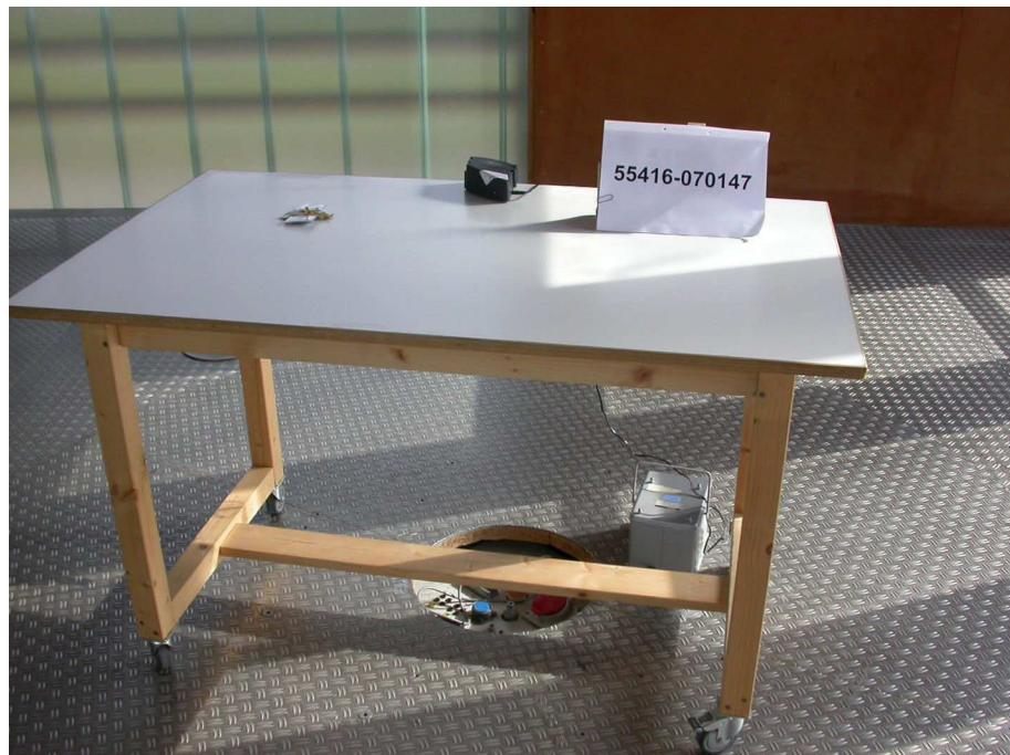
**Test setup for radiated emission measurement
