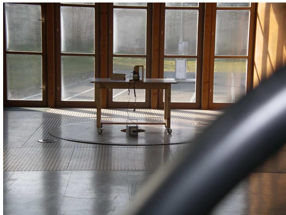
**Test setup for radiated emission measurement
