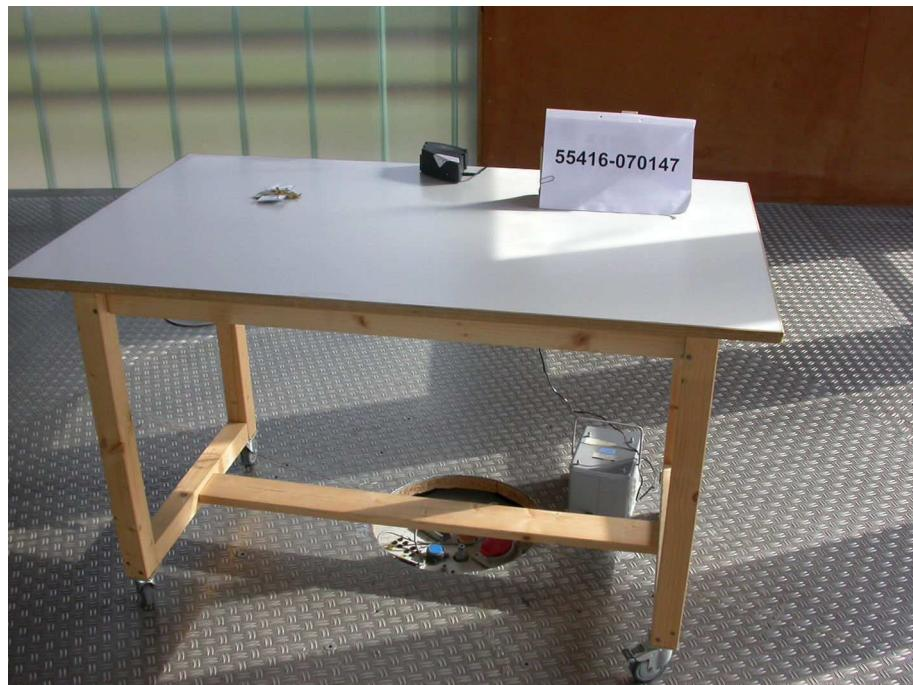
**Test setup for radiated emission measurement
