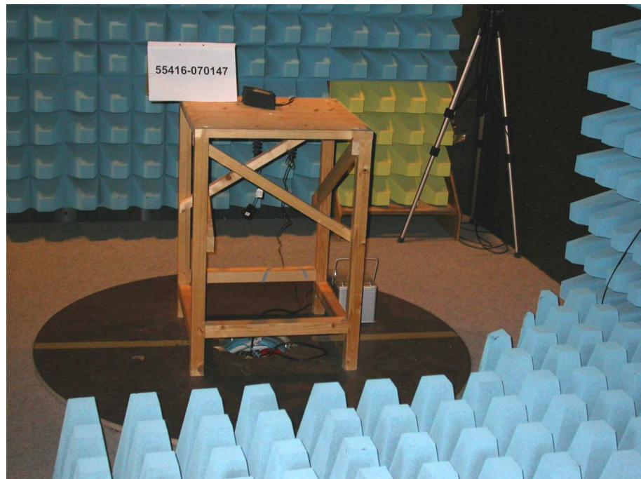
**Test setup for radiated emission measurement
