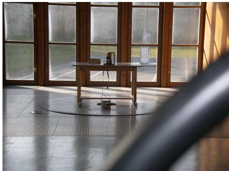
**Test setup for radiated emission measurement
