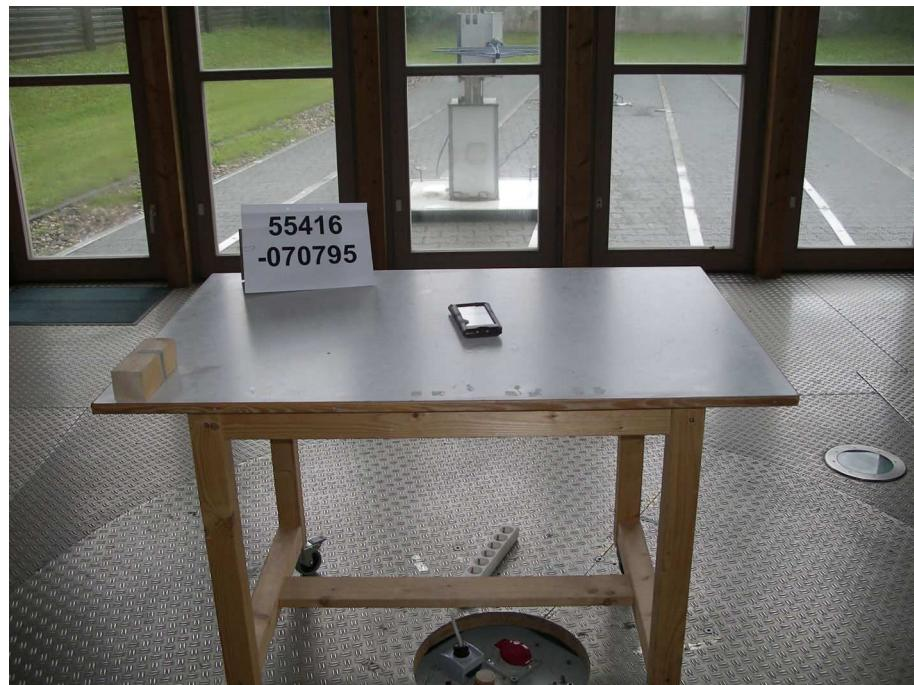
**Test setup for radiated emission measurement
