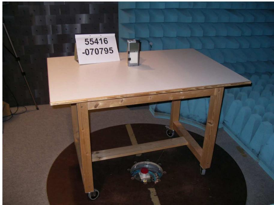
**Test setup for radiated emission measurement
