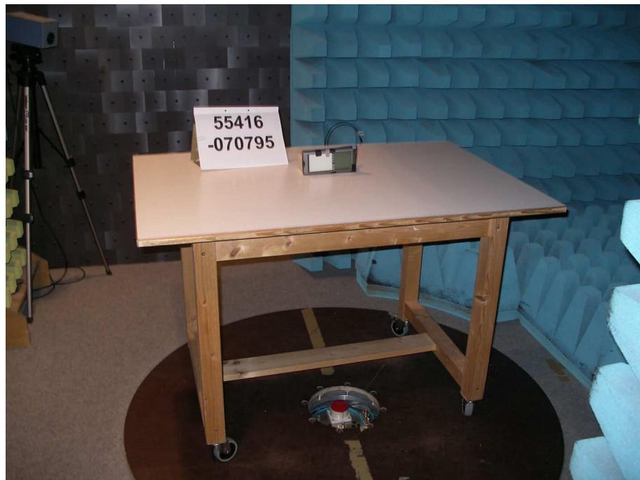
**Test setup for radiated emission measurement
