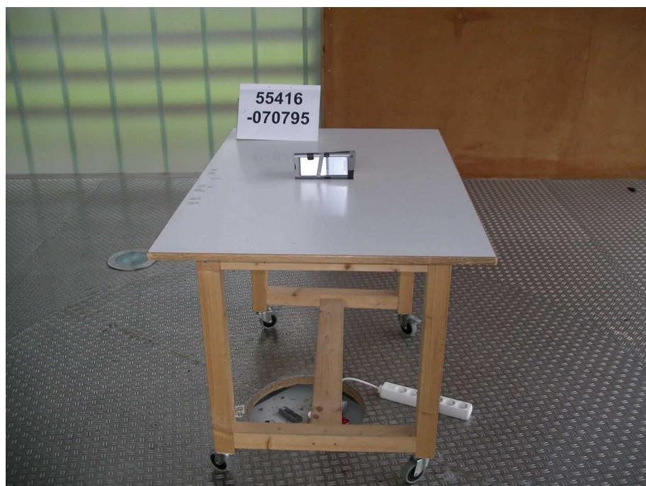
**Test setup for radiated emission measurement
