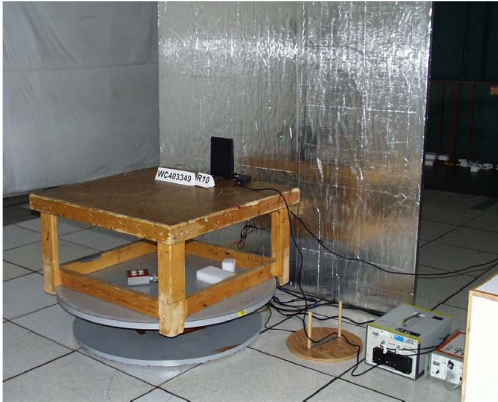
Test-setup photo(s): Conducted emission 10/150 kHz - 30 MHz
