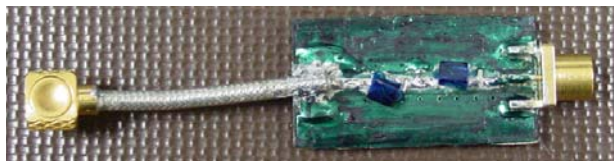
Low Pass Filter Assembly (Top Side)
