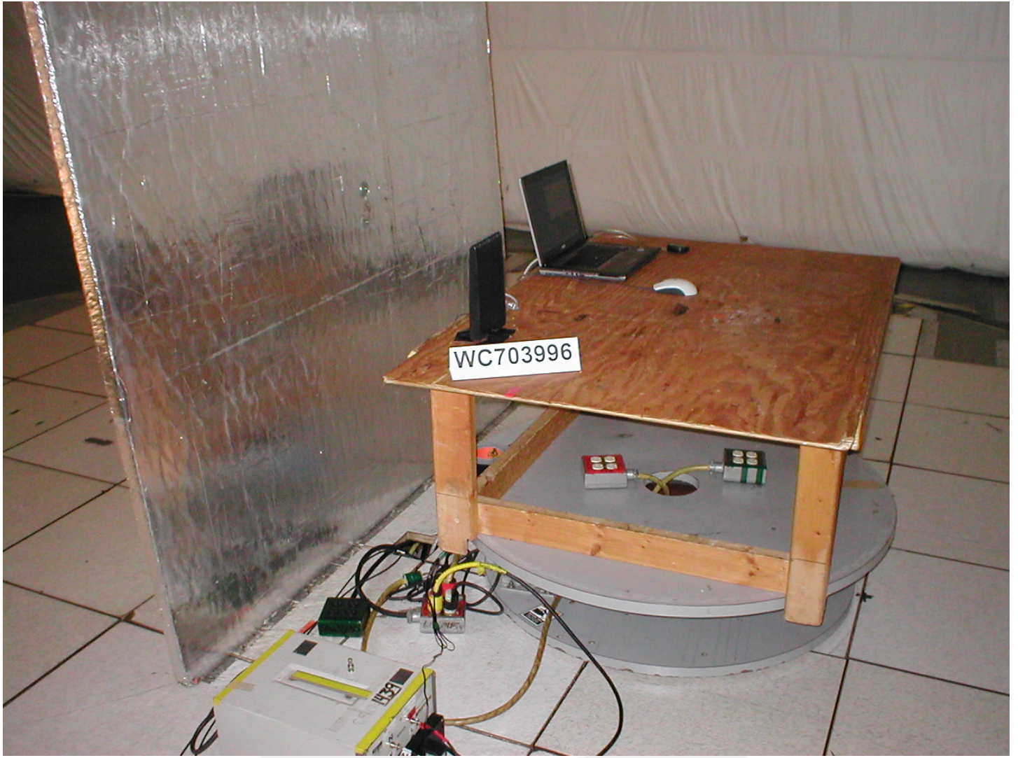
Test setup photo, conducted emissions on AC mains
