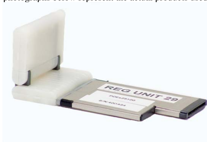
DUT w/ antenna at 90 degrees
