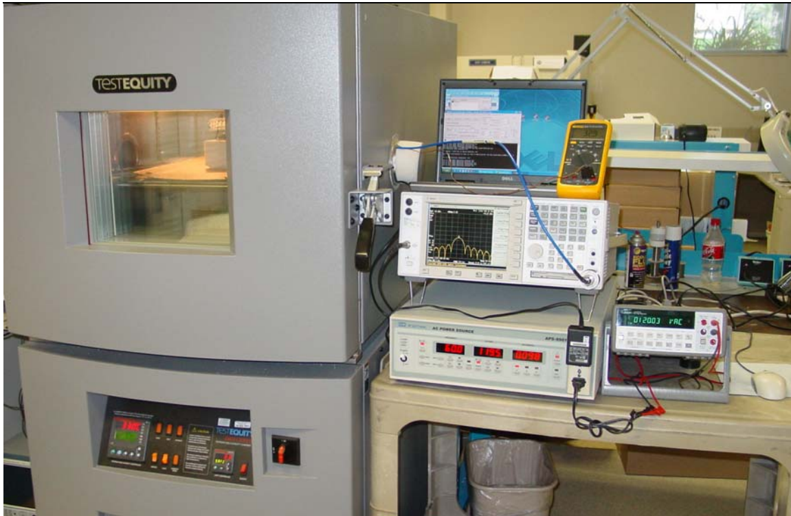
Frequency Stability Test Setup
