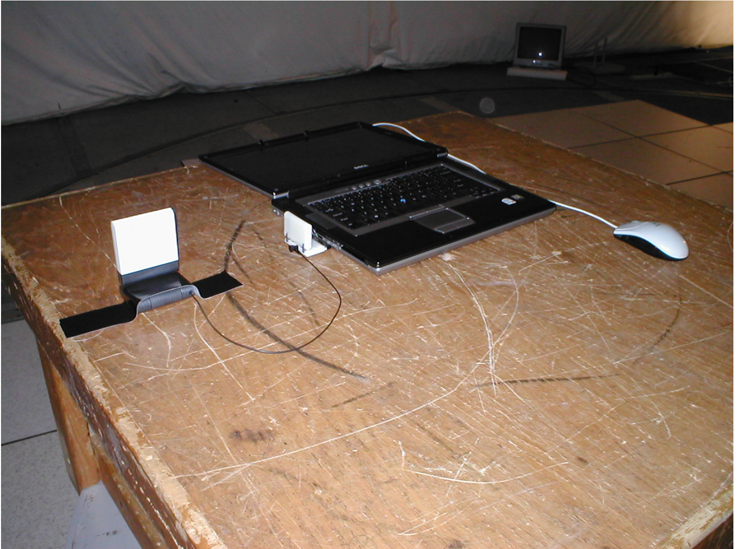
Test setup photo, radiated emissions
