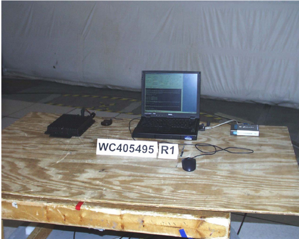
Test-setup photo(s): Radiated emission 30 MHz - 18000 MHz
