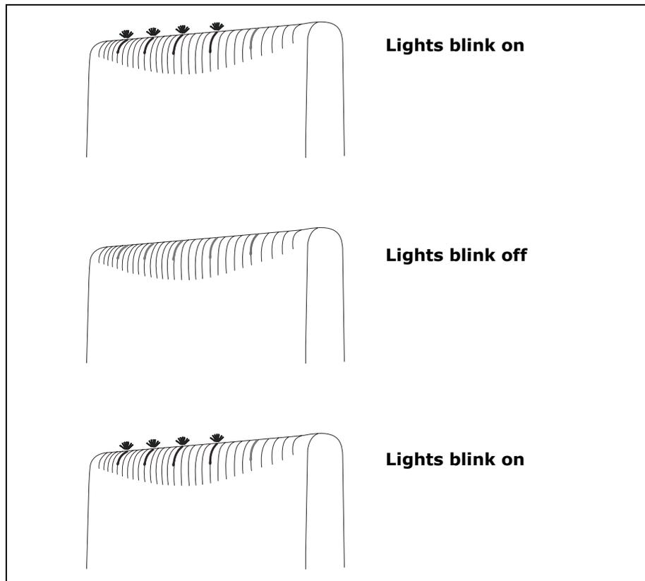
**Figure 7: Indicator lights blinking simultaneously: signal found**
