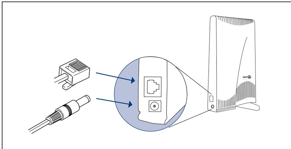
**Figure 2: Ethernet Jack Location on Side of RSU**
