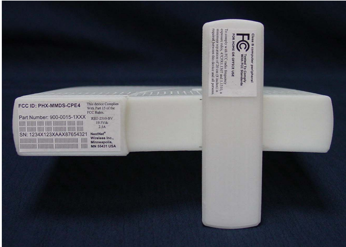
Photo showing label locations on indoor CPE unit
