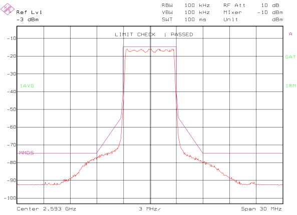
Test Results: Channel 31, 2683 MHz (33dBm / 2W)
