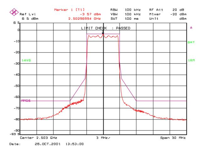
Test Results: Channel 16, 2593 MHz (33dBm / 2W)
