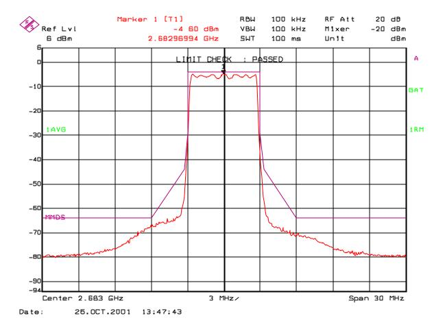
Test Results: Channel 31, 2683 MHz (33dBm / 2W)
