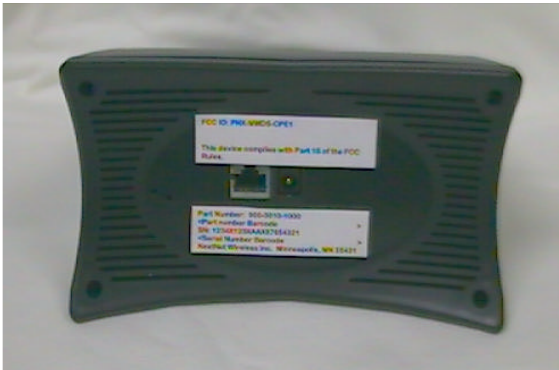
Photo showing label location on CPE unit
