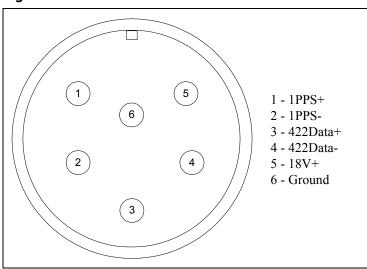
An RS-422 line feeds 1PPS+ and 1PPS- with the time synchronization pulse from the GPS equipment to the base station.
