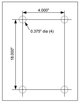
**3** To attach the base station to a wall, use the mounting brackets. Install them on the base station first, then attach the brackets to the wall. To attach the brackets to the base station, use 5/16 inch x 18 inch UNC thread bolts and a lock washer. Use your own bolts to then attach the bracket to the surface.
