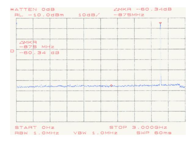
Name of Test: Spurious emissions at antenna terminals
