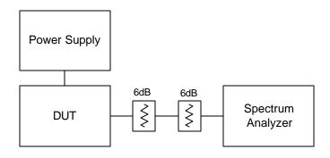
Name of Test: Spurious emissions at antenna terminals
