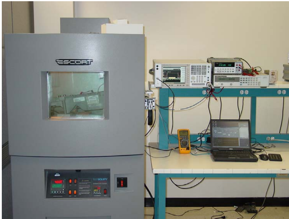
Frequency Stability Test Setup (Outside Chamber)
