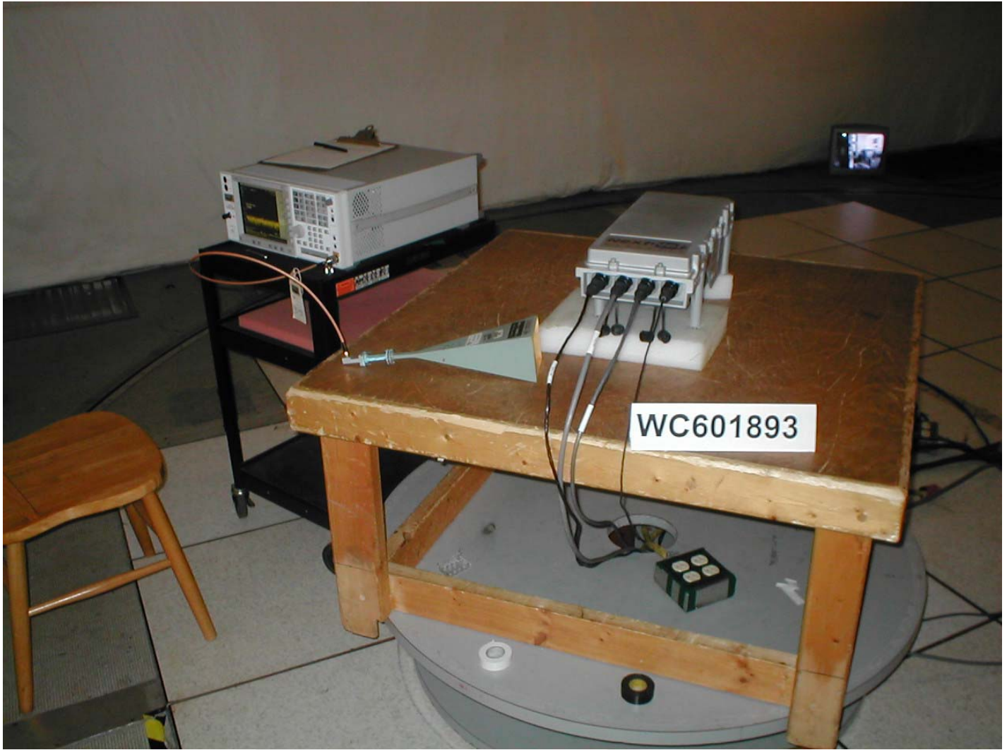
Test setup photo, radiated emissions
