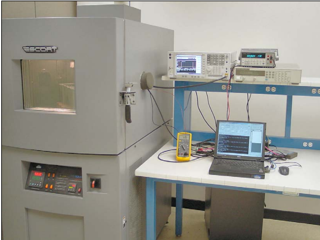
Frequency Stability Test Setup
