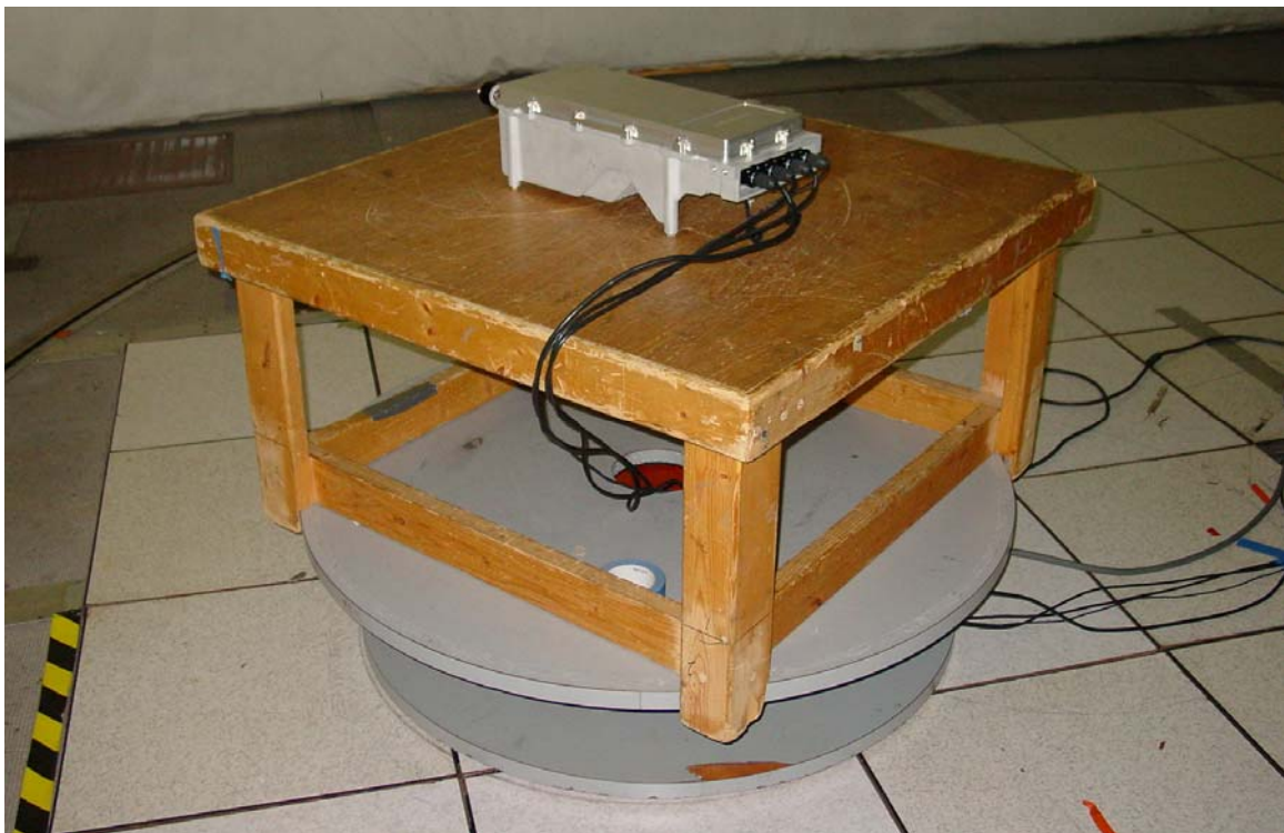
Field Strength of Spurious Radiation (Back View)
