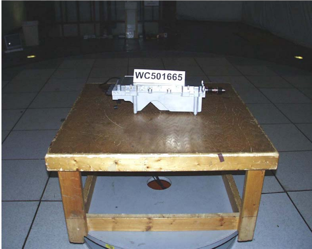
Test-setup photo(s): Radiated emission 30 MHz - 26000 MHz
