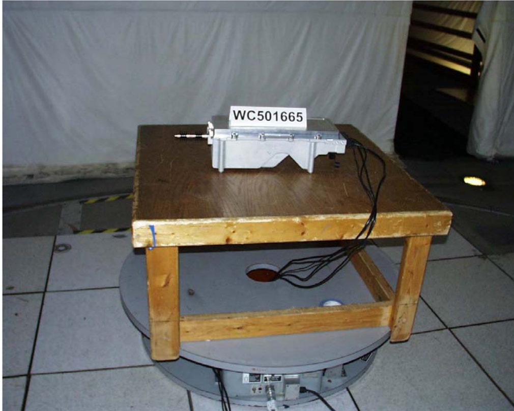
Test-setup photo(s): Radiated emission 30 MHz - 26000 MHz
