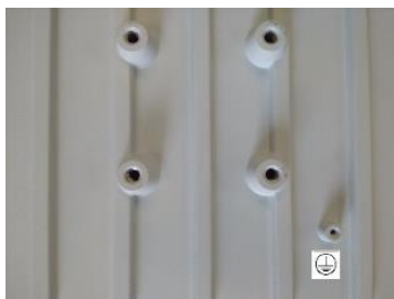
Figure 3-5: Enclosure Ground Connection
