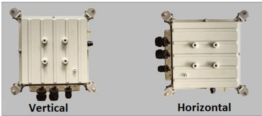
Figure 5-2: ODU Polarization Directions
