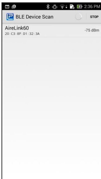
4. The application will scan for AireLink radios. Wait until the scanning finishes.
