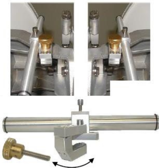
Figure 5-13: Re-configuring Alignment Sight Tool
