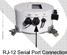
Figure 3-7: ODU Serial Port Connector
