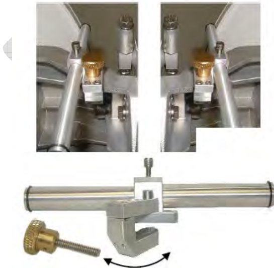
Figure 5-6: Re-configuring Alignment Sight Tool
