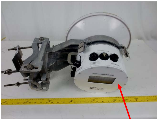
EUT with 1 ft., 45 dBi Antenna
