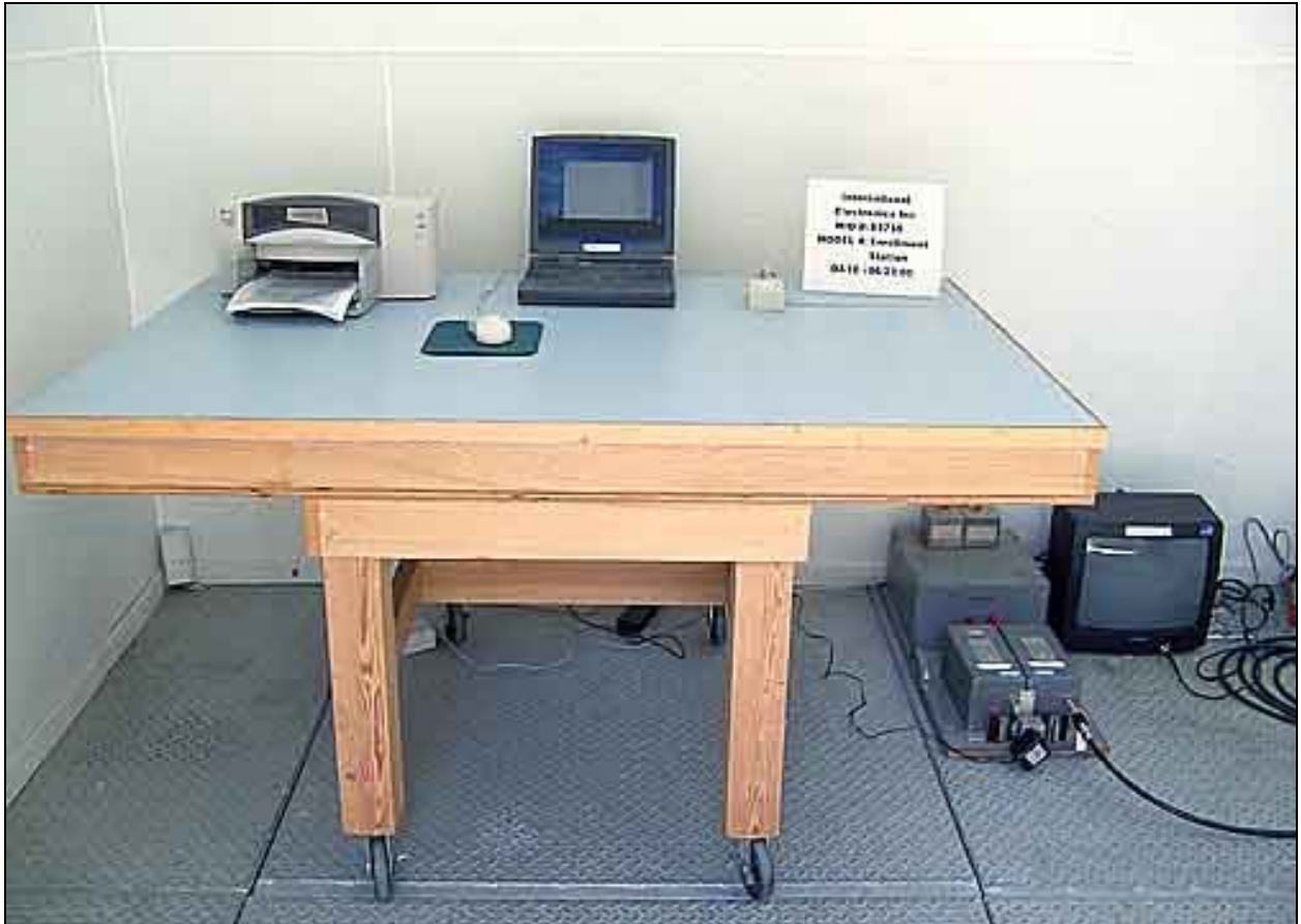
Mains Conducted Emissions - Front View
