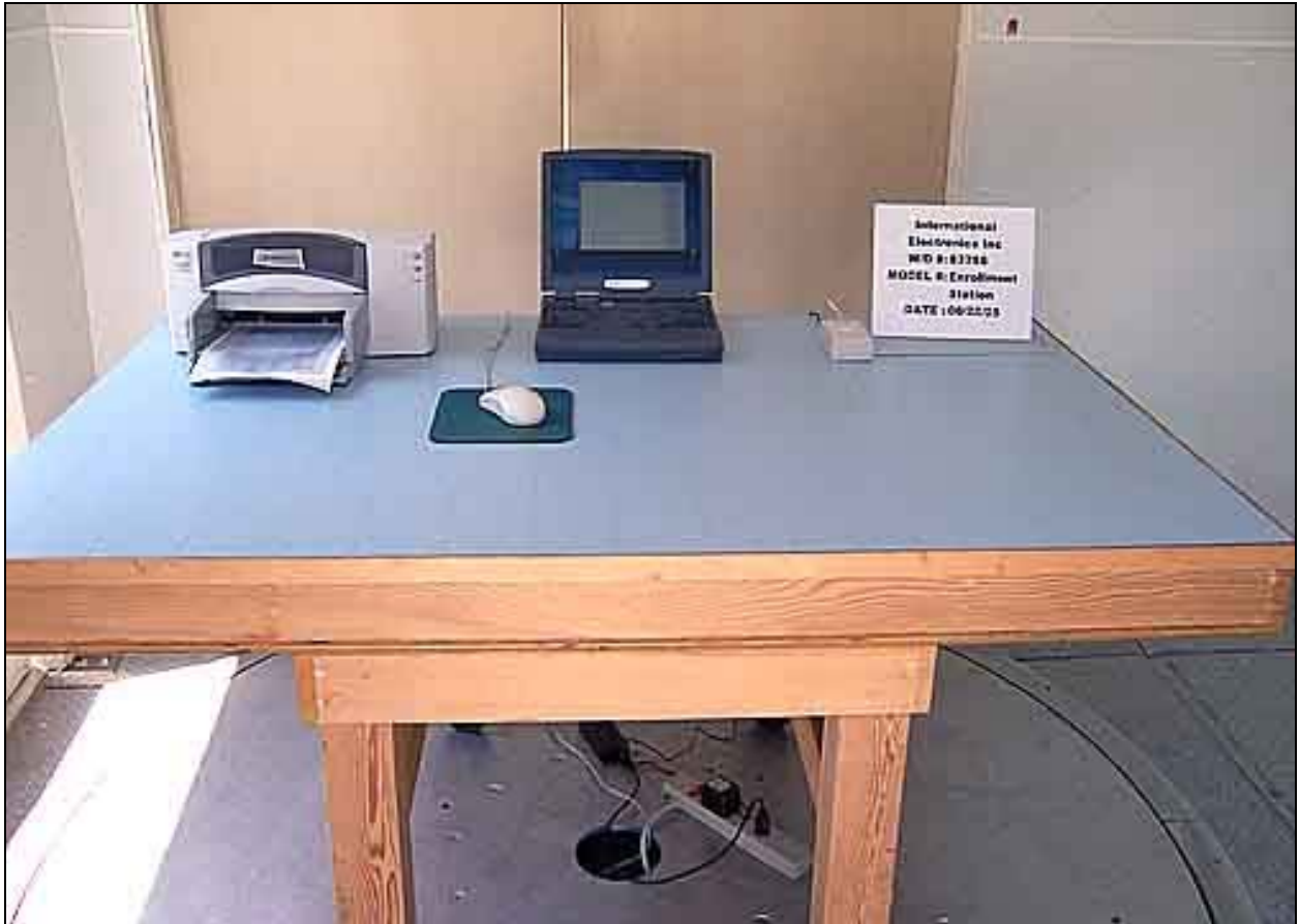
Radiated Emissions - Front View
