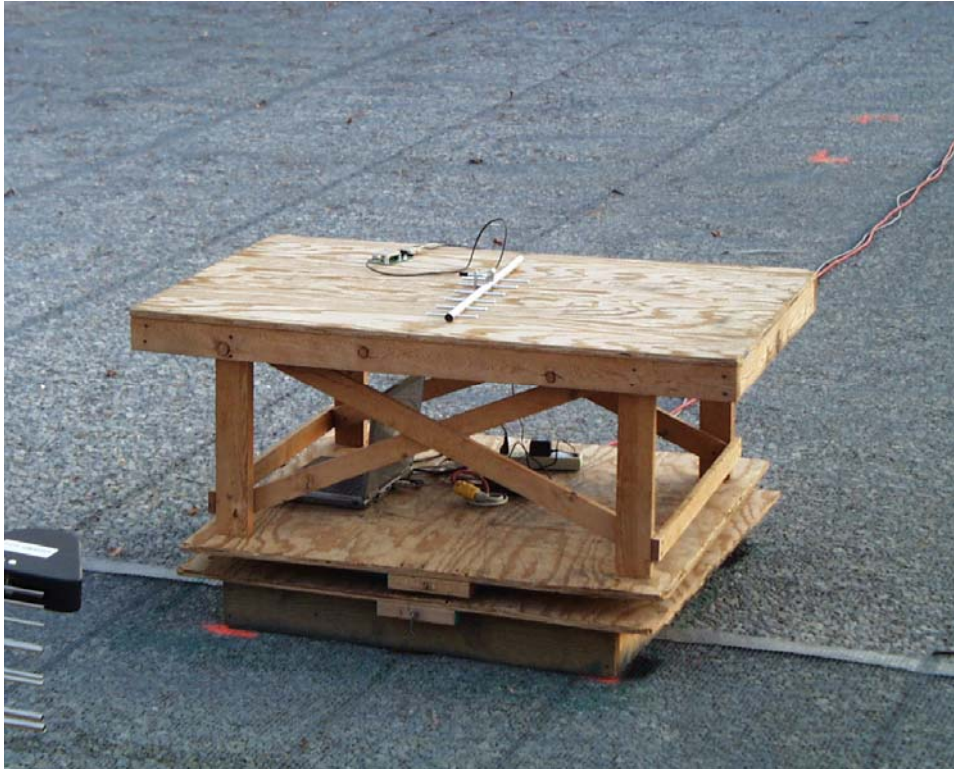
Radiated Emissions Test setup photographs with 6dBi Gain antenna (part number YS8966).
