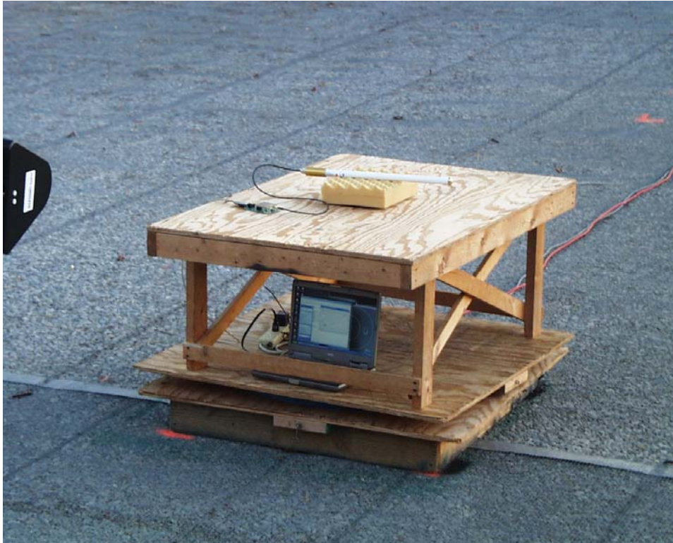
Radiated Emissions Test setup photographs with 3dBi Gain antenna (part number FG8963).
