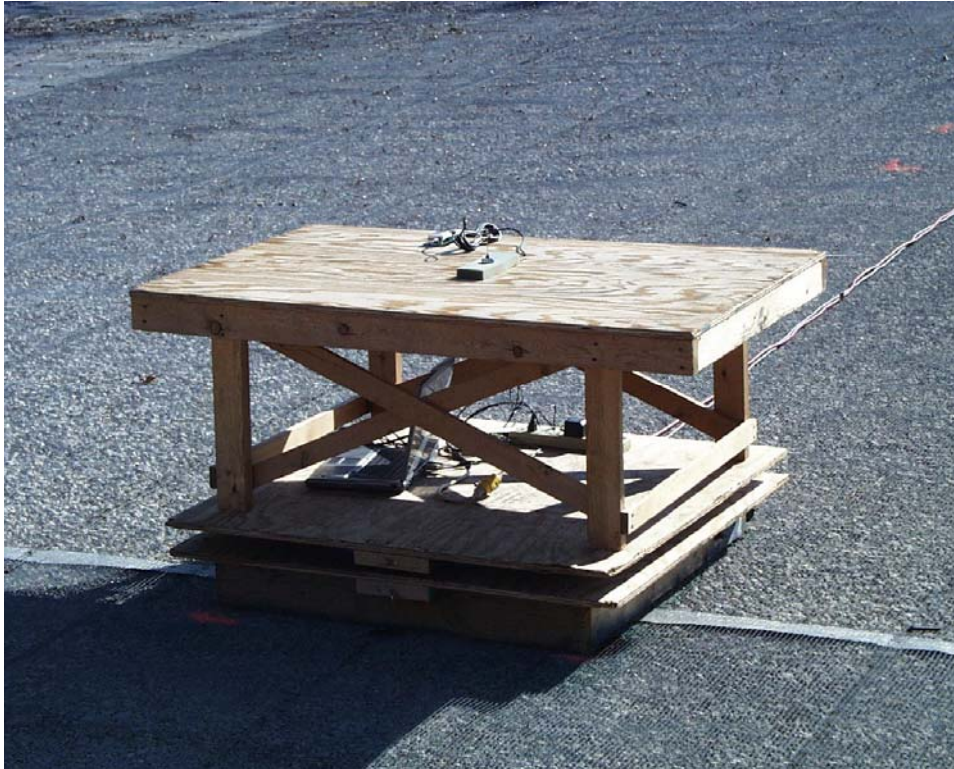
Radiated Emissions Test setup photographs with \frac{1}{4} wave Mobile antenna. (Part number MUF9000)
