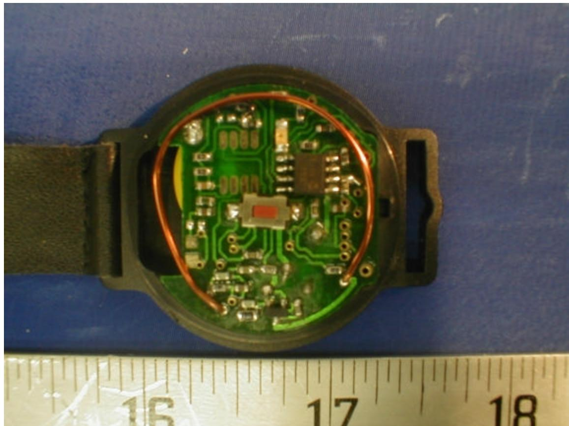
**EUT Circuit Board Solder View**
