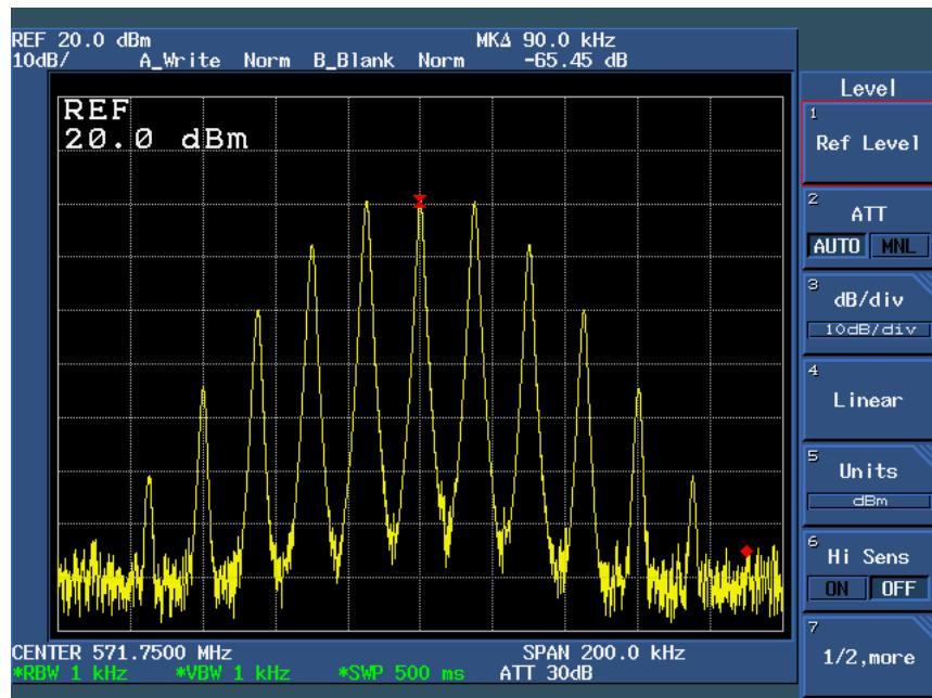
OCCUPIED BANDWIDTH—POWER OUTPUT = 1250 Watts
