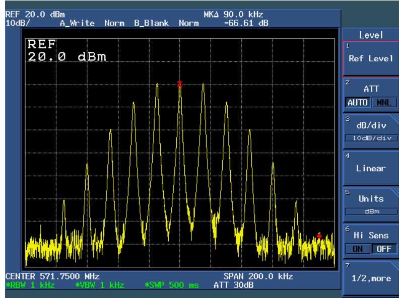
OCCUPIED BANDWIDTH—POWER OUTPUT = 875 Watts Visual, 87 Watts Aural
