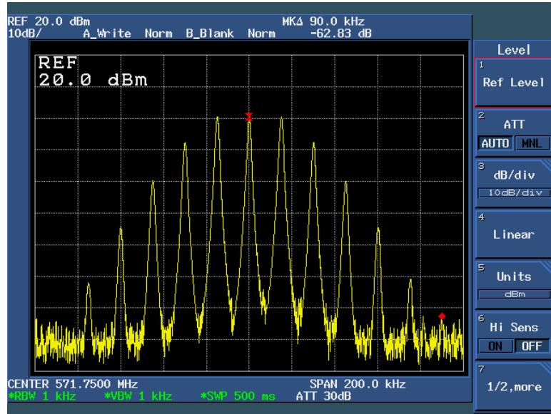
OCCUPIED BANDWIDTH—POWER OUTPUT = 62.5 Watts Visual, 6.25 Watts Aural
