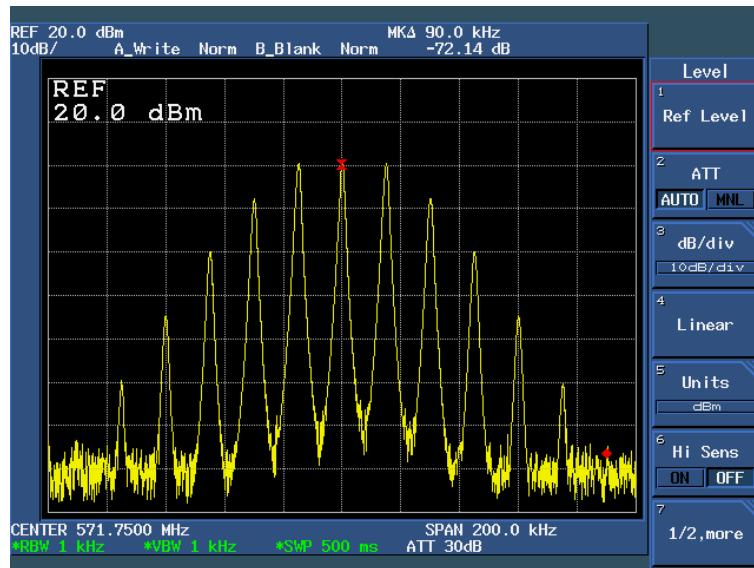
OCCUPIED BANDWIDTH—POWER OUTPUT = 325 Watts Visual, 32.5 Watts Aural
