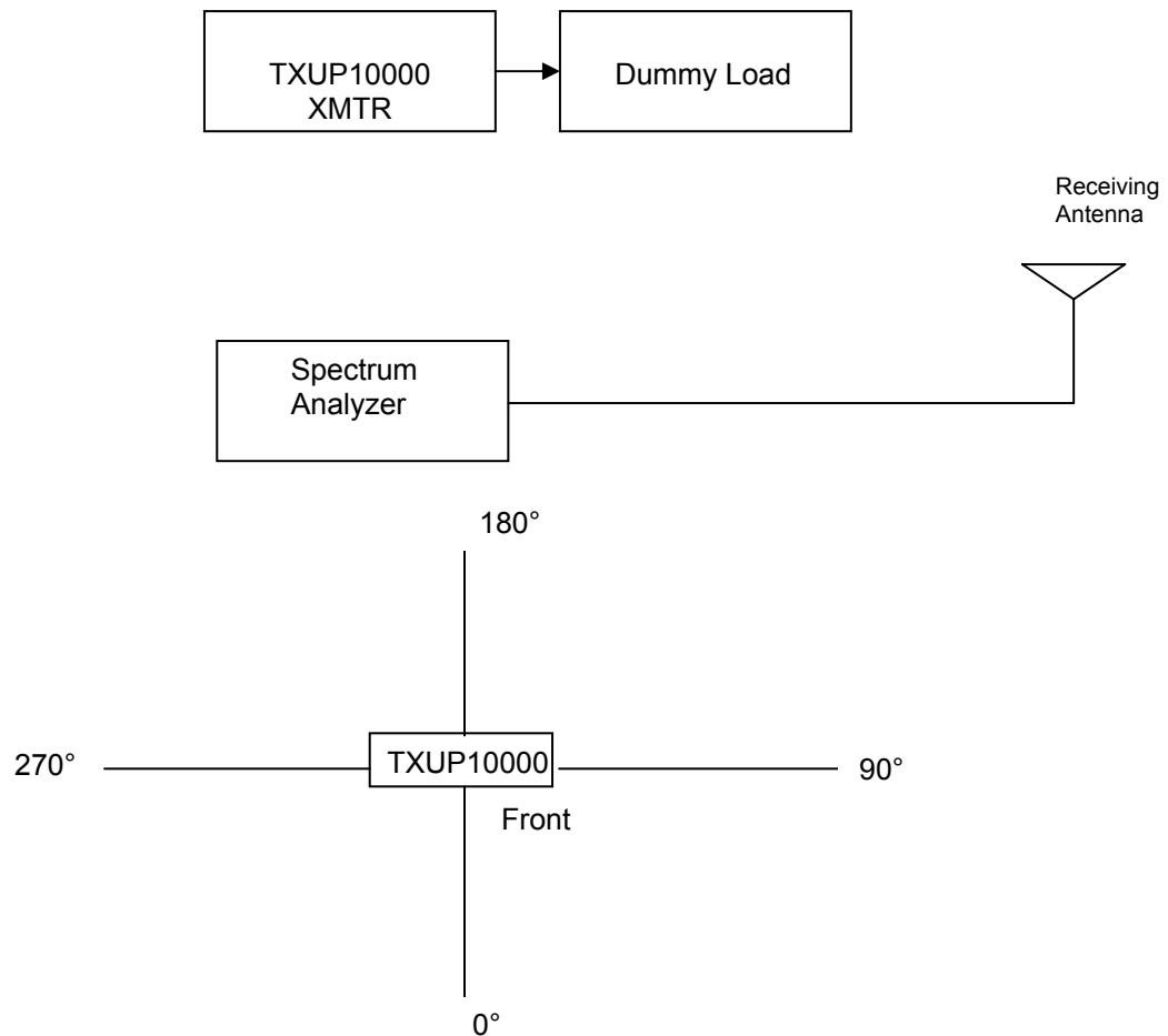
As indicated in the spreadsheet data, the worst case calculation was 79.6 dB at the tenth harmonic. The main limitation is the noise floor of the spectrum analyzer. The measurement tables for the all views of the transmitter at each frequency are shown below. The results indicate that all radiated harmonics meet the FCC requirement of 60 dB as outlined in FCC rule 2.1053 and 2.1057.
