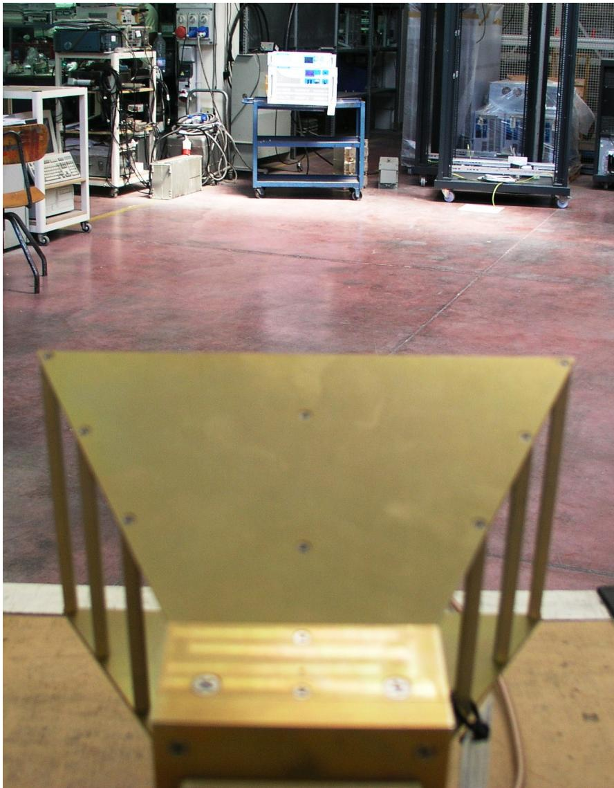
As calculated from the spreadsheet data on the following page, the worst case measurement was 63 dB at the second harmonic (The photo above shows this particular measurement). The measurement tables for the remaining views of the transmitter are shown on the following pages.
