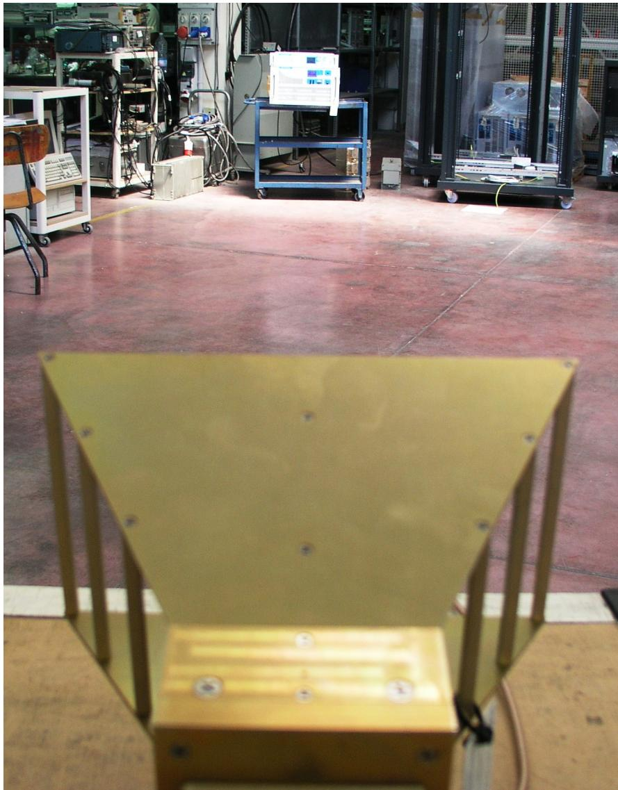
As calculated from the spreadsheet data on the following page, the worst case measurement was -75 dB at the second harmonic (The photo above shows this particular measurement). The measurement tables for the remaining views of the transmitter are shown on the following pages.
