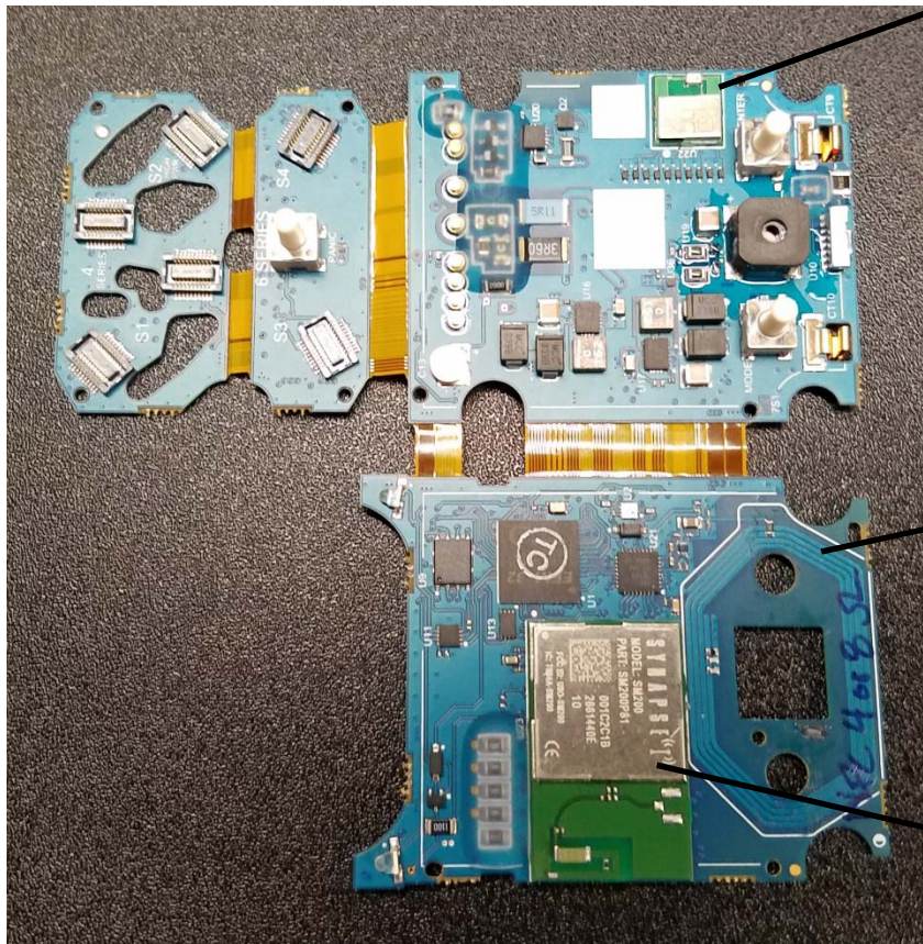
View of circuit board w/o sensors or plastic carrier (side 1)
