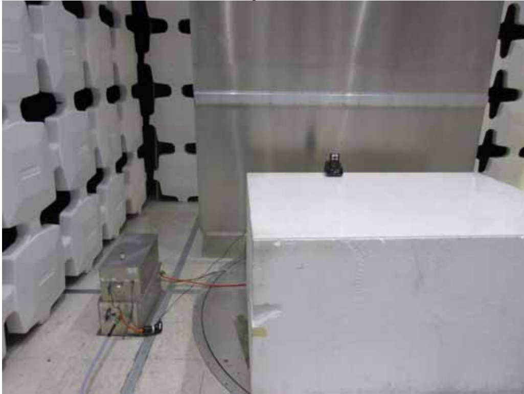
Test Setup for Power Line Conducted Emissions Tests
