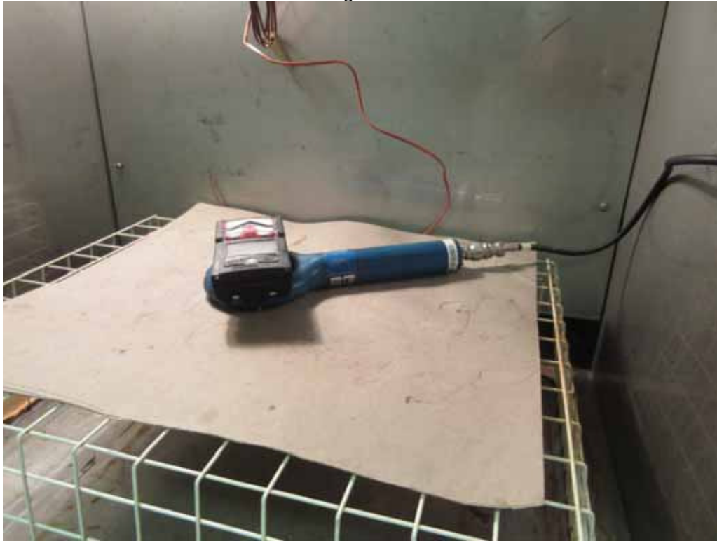
Test Setup for Frequency Stability Tests
