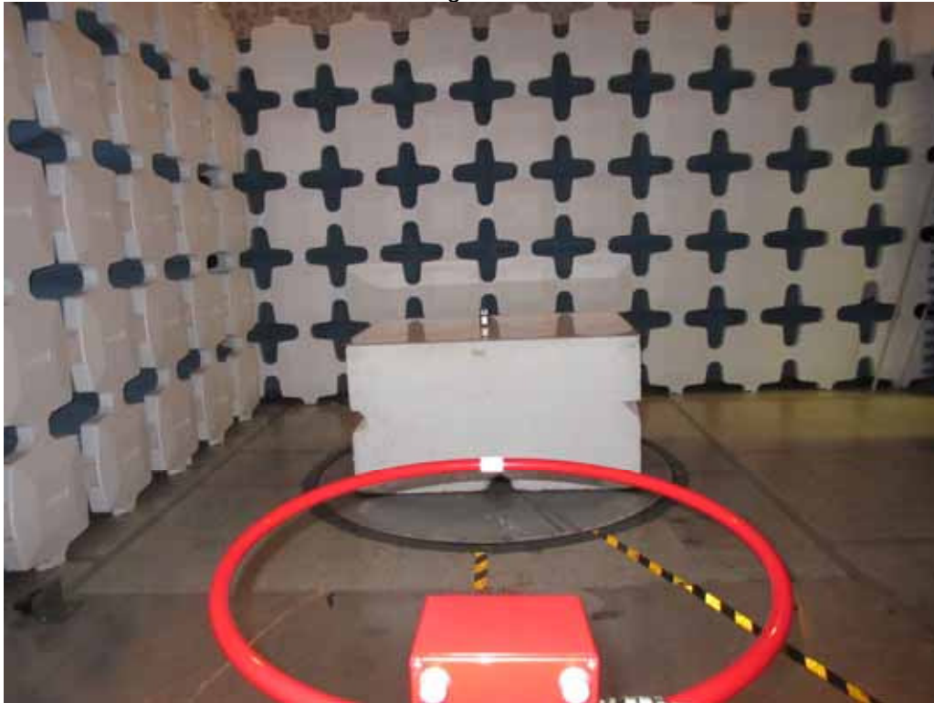
Test Setup for Radiated Emissions below 30MHz – Horizontal Polarization
