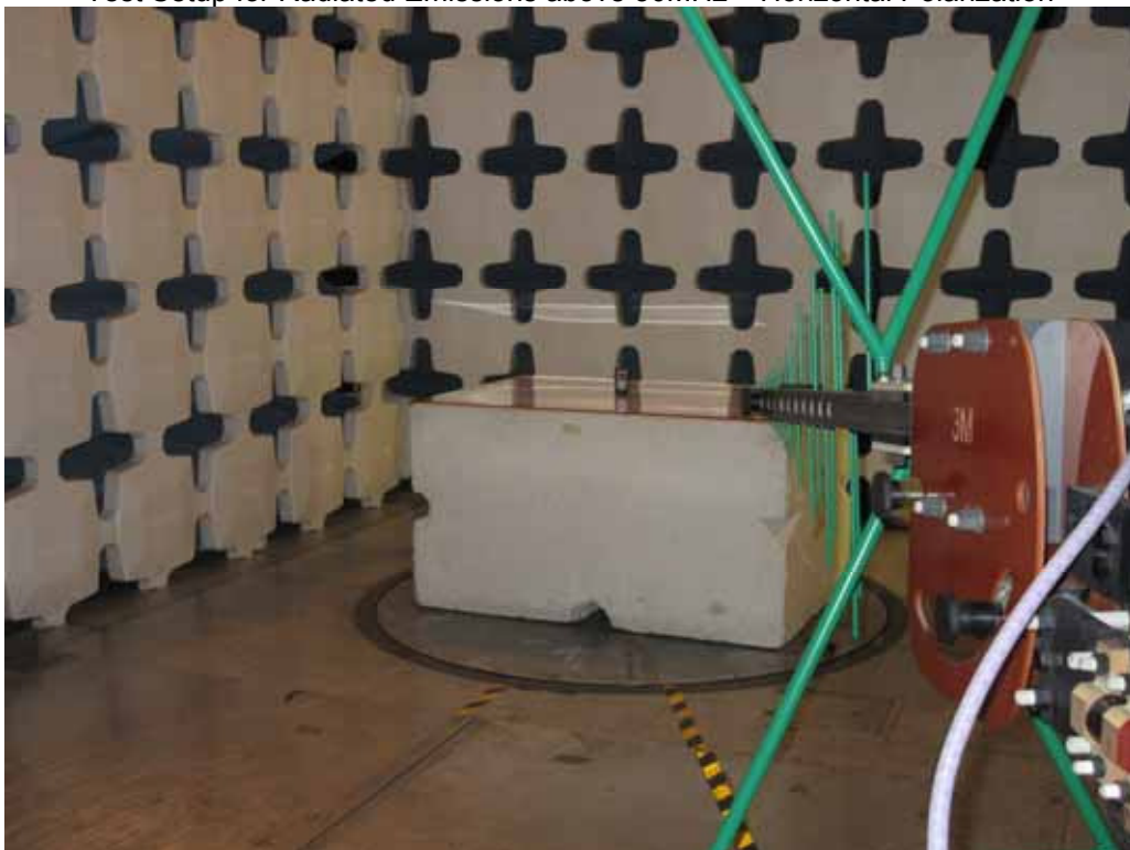
Test Setup for Radiated Emissions above 30MHz – Vertical Polarization
