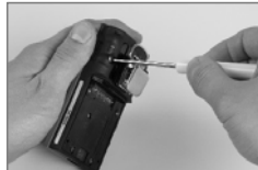
Using a torx screwdriver, loosen the remaining two screws from the case bottom.
