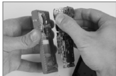
Hold the plastic sides that border the sensors near the top of circuit board assembly. Gently lift the circuit board assembly straight away from
