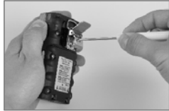
Use a Philips screwdriver to access the clip's screw. Turn counterclockwise to loosen and remove the screw and washer.
