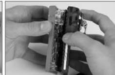
Hold the case bottom near the upper screws. Lift the case top slightly to separate the top and bottom.
