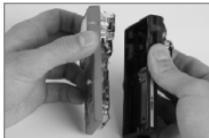
Continue to lift the case top straight up to remove it.
