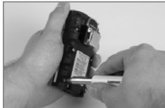
Using a torx screwdriver, loosen all four screws on the battery pack.
