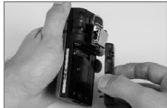
Lift the battery pack away from the instrument.
