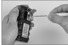
Guide the screwdriver through the clip's hole and into the screw head. Turn clockwise to tighten.
