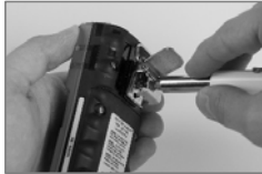
To attach the clip, place the screw through the center hole of the clip back.
