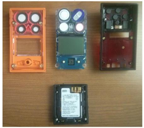
2. Shown below is the PCBA with LCD and sensors removed and PCBA removed from its plastic frame. The NFC shield (black, bottom left) is shown applied to the PCB antenna.
