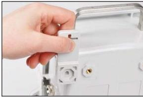
Using the orientation shown, mate the hexagon cutout of the wall mount to a corresponding corner on the back of the RGX. The cross portion will extend past the edge of the case.
