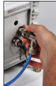
Turn the IS power port cap counterclockwise (approximately 45°) to expose the port for use.
