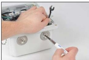
Hold the hex nut in place with a 3/8 " open-end wrench and turn the T20 torx screw clockwise to tighten.
