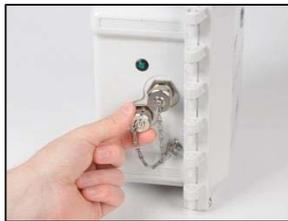
Uncap the unit's charging power supply port: turn the port cap counterclockwise to expose the port for use.
