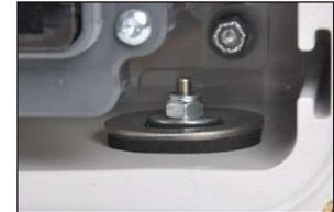
Follow with the sealing gasket, flat washer, and hex nut.
