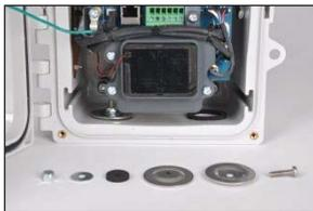
Remove the nut, two internal washers, the sealing gasket, and one external washer from the case.
