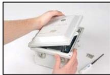
Using a torx screwdriver with a T25 bit, unscrew and remove the four screws that secure the case lid to the case base.
