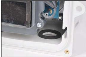
Remove the protective paper to expose the adhesive side of the gasket.
