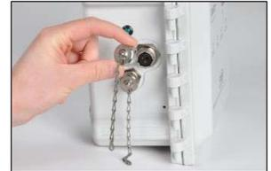
To remove a worn or damaged port cap, locate the hex nut for the tethered-chain screw inside the case.
