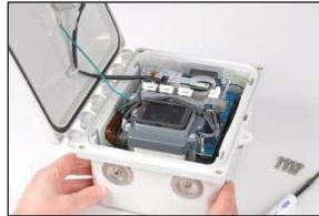
When closing the lid, ensure all wires and cables are secure and are contained inside the case, away from its closure surfaces.
