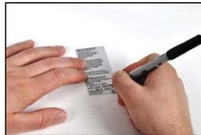
Locate the unit's LAN MAC and WAN MAC values, which are included on the label that is factory affixed to the back of the unit. Record these two values onto the kit label in the areas provided.
