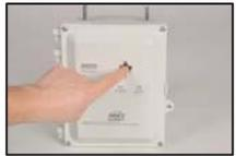
Before connecting the Ethernet cable, you will need to ensure the computer and the RGX are on the same network. Consult your network administrator for assistance. *Note:* For network connections, the RGX default static IP is 192.168.1.1.
