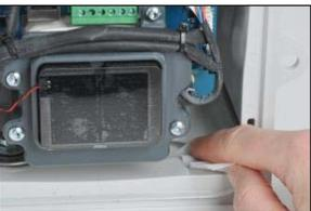
Use the glue side of the removed gasket in a dabbing motion to lift off remaining adhesive.
