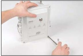
Use a T25 torx screwdriver to unscrew and remove the four fasteners that secure the case lid to the case base; set aside the screws for later reinstallation.
