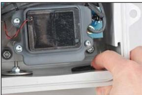
To remove a worn or damaged fixed gasket, push the outer edge of the gasket toward its center with a finger; use friction and a forward motion to separate the gasket from the base.
