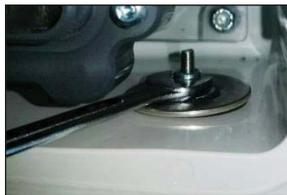
Inside the case, hold the nut in place with a 3/8 " open-end wrench and turn the T20 torx screw counterclockwise to loosen.
