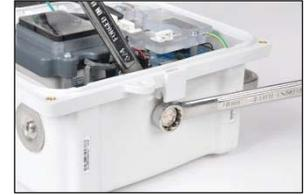
To remove the vent, use an 18 mm open-end wrench to hold the vent in place.
