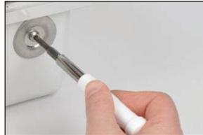
From outside of the case, place the torx screw into the concave side of the washer, and place over the base opening.
