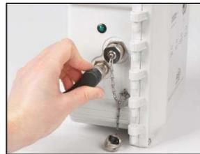
Connect the power-supply cable to the port and turn its swivel cover clockwise (approximately 45°) until it clicks closed or a full-stop connection feedback is felt.
