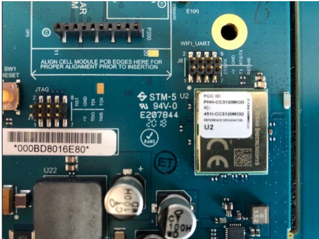
Picture of the new PHH-CC3120MOD FCC ID placed onto the module
