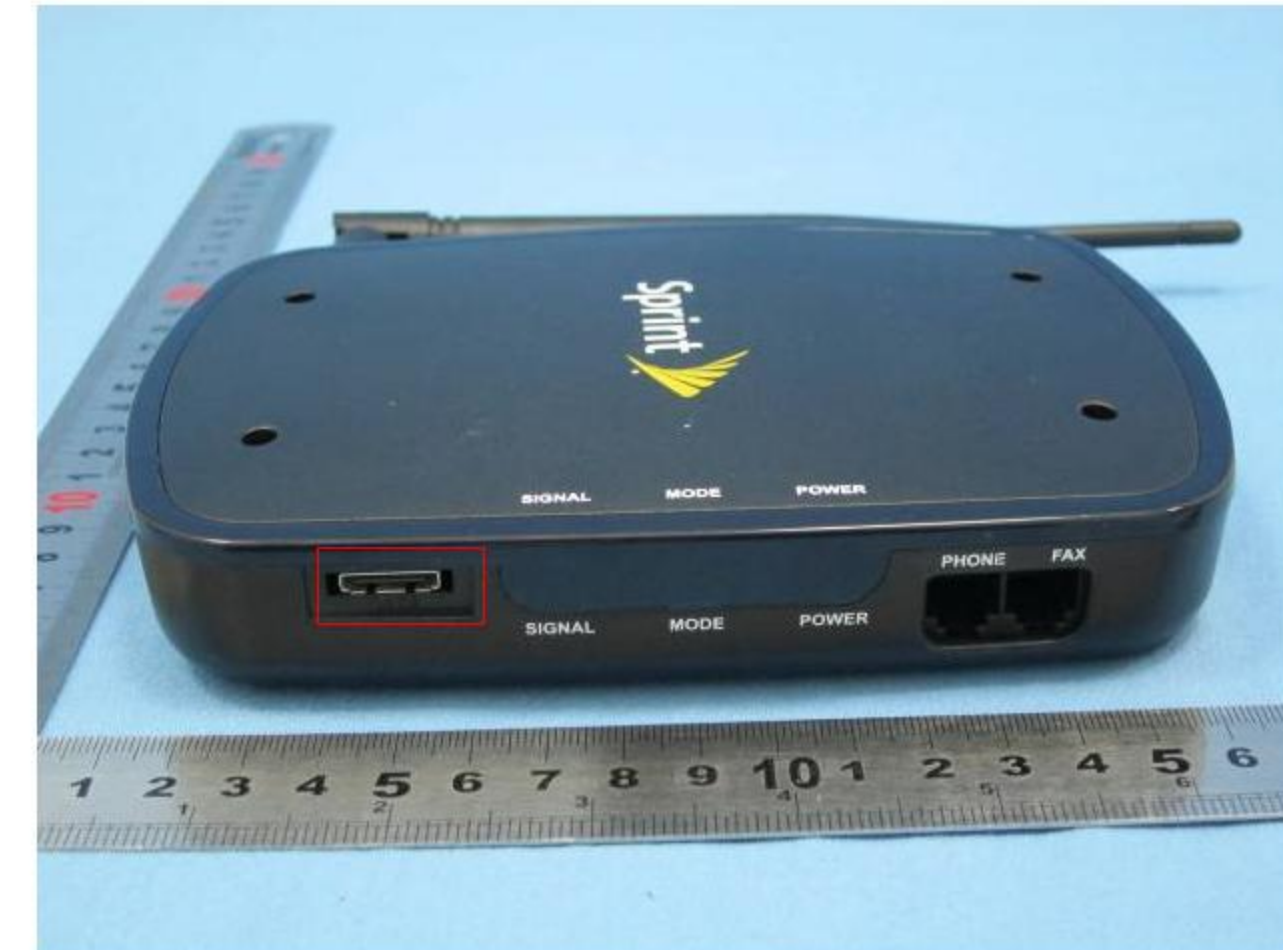
Note: the red part is the port only for engineering test use but the ender user will not use.
