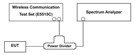
(Configuration of conducted Emission measurement) Test Procedure
