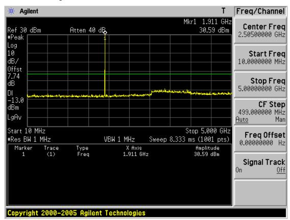
Spurious Emissions at Antenna Terminal / Ch.810 -1
