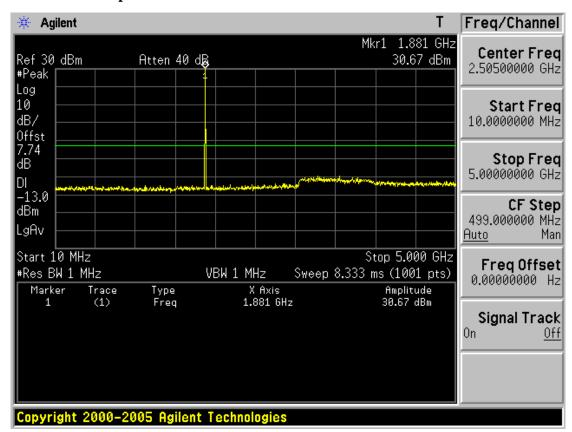
PCS1900 Spurious Emissions at Antenna Terminal / Ch.661 -1
