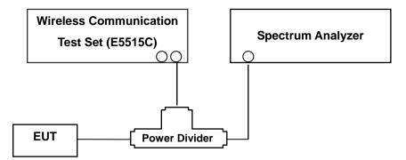
(Configuration of conducted Emission measurement) Test Procedure
